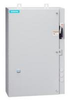
Non-reversing motor starter, Size 2 1/2, Three phase full voltage, Solid-state overload relay, OLR amp range 25-100A, Combination type, 100A circuit breaker, Enclosure NEMA type 4/12, Water/dust tight for outdoors, Extra-wide enclosure
