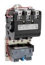
Non-reversing motor starter Size 2 1/2 Three phase full voltage Solid-state overload relay OLRelay amp range 25-100A 550/575-600 50/60HZ coil Combination type No enclosure
