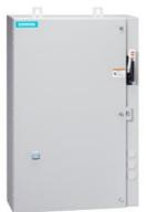
Non-reversing motor starter, Size 2 1/2, Three phase full voltage, Solid-state overload relay, OLR amp range 25-100A, Combination type, 100A fusible disconnect, 100A/600V fuse clip, Encl NEMA type 4X 304 S-Steel, Water/dust tight noncorrosive, Standard width enclosure
