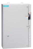
Non-reversing motor starter, Size 3, Three phase full voltage, Solid-state overload relay, OLR amp range 25-100A, 208VAC 60Hz coil, Combination type, 125A circuit breaker, Enclosure NEMA type 4/12, Water/dust tight for outdoors, Extra-wide enclosure
