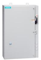
Non-reversing motor starter, Size 2, Three phase full voltage, Solid-state overload relay, OLR amp range 13-52A, 24VAC 50-60Hz coil, Combination type, 50A circuit breaker, Encl NEMA type 4X 316 S-Steel, Water/dust tight noncorrosive, Extrawide enclosure
