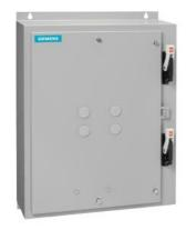
Duplex starter w/o alternator Size 3.5 Three phase full voltage Solid-state overload relay OLR amp range 50-200A Combination type Two 200A disconnect switches Encl NEMA type 4X 304 S. Steel Water/dust tight non-corrosive
