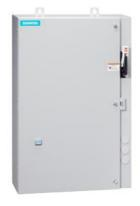
Non-reversing motor starter, Size 2 1/2, Three phase full voltage, Solid-state overload relay, OLR amp range 25-100A, Combination type, 100A fusible disconnect, 100A/250V fuse clip, Encl NEMA type 4X 304 S-Steel, Water/dust tight noncorrosive, Standard width enclosure
