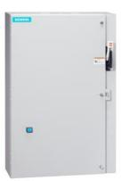
Non-reversing motor starter, Size 4, Three phase full voltage, Solid-state overload relay, OLR amp range 50-200A, 110V 50Hz / 120V 60Hz coil, Combination type, 150A circuit breaker, Enclosure NEMA type 1, Indoor general purpose use, Standard width enclosure
