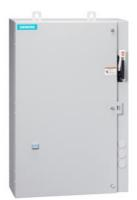
Non-reversing motor starter Size 3 Three phase full voltage Solid-state overload relay OLRelay amp range 25-100A 24VAC 50-60HZ coil Combination type 100A non-fusible disconnect Encl NEMA type 4X 316 S-steel Water/dust tight non-corrosive Standard width enclosure
