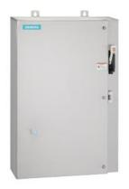
Non-reversing motor starter, Size 4, Three phase full voltage, Solid-state overload relay, OLR amp range 50-200A, 208VAC 60Hz coil, Combination type, 200A nonfusible disconnect, Encl NEMA type 4X 304 S-Steel, Water/dust tight noncorrosive, Standard width enclosure
