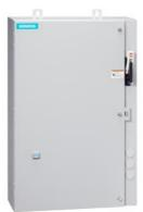
Non-reversing motor starter, Size 3, Three phase full voltage, Solid-state overload relay, OLR amp range 25-100A, Combination type, 125A circuit breaker, Enclosure NEMA type 4/12, Water/dust tight for outdoors, Extra-wide enclosure
