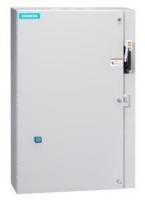
Non-reversing motor starter, Size 3, Three phase full voltage, Solid-state overload relay, OLR amp range 25-100A, Combination type, 125A circuit breaker, Enclosure NEMA type 1, Indoor general purpose use, Extra-wide enclosure
