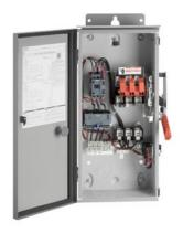
Slim Line Pump Control Panel NEMA size 1 Three phase full voltage Solid-state overload relay OLR amp range 10-40A 220/230V 50/60Hz Coil 30A fusible disconnect 30A/250V fuse clip 1NC / 1NO auxiliary contacts HOA Sel. Sw. <(>&<)> Start/Stop 3-point power terminal block 3-point control terminal block 3-point ground lug Enclosure NEMA type 3/3R Weather proof outdoor use
