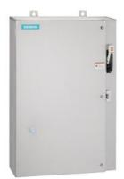
Non-reversing motor starter, Size 2 1/2, Three phase full voltage, Solid-state overload relay, OLR amp range 25-100A, 240V 50Hz / 277V 60Hz coil, Combination type, 100A circuit breaker, Encl NEMA type 4X 316 S-Steel, Water/dust tight noncorrosive, Extra-wide enclosure
