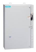
Non-reversing motor starter Size 0 Three phase full voltage Solid-state overload relay OLRelay amp range 0.75-3.4A 24VAC 50-60HZ coil Combination type 3Amp circuit breaker Encl NEMA type 4X 316 S-steel Water/dust tight noncorrosive Extra-wide enclosure
