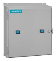
Duplex starter w/o alternator, Size 2, Three phase full voltage, Solid-state overload relay, OLR amp range 13-52A, 208VAC 60Hz coil, Non-combination type, Encl NEMA type 4X 304 S-Steel, Water/dust tight noncorrosive
