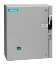
Non-reversing motor starter Size 3 Three phase full voltage Solid-state overload relay OLRelay amp range 25-100A 208VAC 60HZ coil Combination type 125Amp circuit breaker Enclosure NEMA type 1 Indoor general purpose use Standard width enclosure
