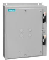
Duplex starter w/o alternator Size 1.75 Three phase full voltage Solid-state overload relay OLR amp range 10-40A 24VAC 50-60Hz Coil Combination type Two 60A disconnect switches Encl NEMA type 4X 304 S. Steel Water/dust tight non-corrosive
