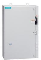
Non-reversing motor starter Size 0 Three phase full voltage Solid-state overload relay OLRelay amp range 3-12A 190-220/220-240V 50/60HZ coil Combination type 10Amp circuit breaker Encl NEMA type 4X 316 S-steel Water/dust tight noncorrosive Extra-wide enclosure
