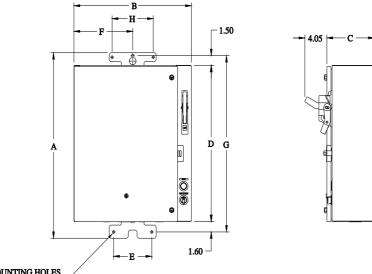
MOUNTING HOLES FOR <sup>5</sup>/<sub>16</sub>" HARDWARE
