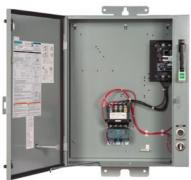
Pump control panel, Size 1, Three phase full voltage, Solid-state overload relay, OLR amp range 5.5-22A, 240V 50Hz / 277V 60Hz coil, Standard type contactor, 25A circuit breaker, HOA Sel Sw. <(>&<)> Start P.B., Enclosure NEMA type 3/3R, Weather proof outdoor use
