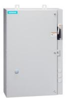
Non-reversing motor starter, Size 1, Three phase full voltage, Solid-state overload relay, OLR amp range 0.75-3.4A, 24VDC coil, Combination type, 30A non-fusible disconnect, Encl NEMA type 4X 304 S-Steel, Water/dust tight noncorrosive, Extrawide enclosure
