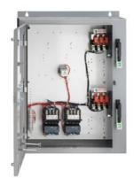
Duplex starter with alternator Size 1.75 Three phase full voltage Solid-state overload relay OLR amp range 10-40A 110VAC 50Hz / 120VAC 60Hz Coil Combination type Two 60A disconnect switches Encl NEMA type 4 painted steel Water/dust tight weather proof
