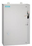
Non-reversing motor starter, Size 4, Three phase full voltage, Solid-state overload relay, OLR amp range 50-200A, 208VAC 60Hz coil, Combination type, 150A circuit breaker, Encl NEMA type 4X 316 S-Steel, Water/dust tight noncorrosive, Standard width enclosure
