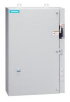
Non-reversing motor starter, Size 0, Three phase full voltage, Solid-state overload relay, OLR amp range 0.75-3.4A, 24VAC 50-60Hz coil, Combination type, 30A fusible disconnect, 30A/600V fuse clip, Encl NEMA type 4X 304 S-Steel, Water/dust tight noncorrosive, Extra-wide enclosure
