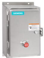
Non-reversing motor starter, Size 0, Three phase full voltage, Solid-state overload relay, OLRelay amp range 3-12a, 110V 50HZ / 120V 60HZ coil, Non-combination type, Enclosure type 4X 304 S-steel, Water/dust tight noncorrosive, Standard width enclosure
