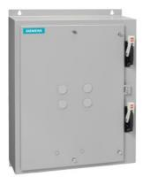
Duplex starter w/o alternator, Size 1 3/4, Three phase full voltage, Solid-state overload relay, OLR amp range 10-40A, 208VAC 60Hz coil, Combination type, Two 40A circuit breakers, Encl NEMA type 4X 304 S-Steel, Water/dust tight noncorrosive
