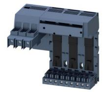
Infeed left Connection main circuit: screw terminal 3 slots for compact load feeders Connection terminal maximum 50 mm2 / 70 mm2
