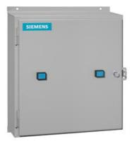
Duplex starter w/o alternator, Size 2 1/2, Three phase full voltage, Solid-state overload relay, OLR amp range 25-100A, 380-440/440-480V 50/60Hz coil, Noncombination type, Enc NEMA type 4 painted steel, Water/dust tight for outdoors
