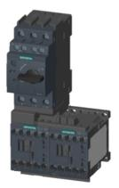
Fuseless motor starter Reversing operation 600VAC Size S00 0.22-0.32a 24V DC screw connection For screw mounting Or 35 mm rail-mounting Type of coordination 2 IQ = 150 KA Also full fills type Of coordination 1 1NO+1NC (MSP) 1NC (per contactor)
