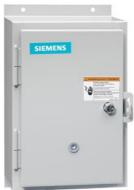
Reversing motor starter, Size 0, Three phase full voltage, Solid-state overload relay, OLR amp range 0.75-3.4A, 110V 50Hz / 120V 60Hz coil, Non-combination type, Enclosure type 12, Dust/drip proof for indoors, Standard width enclosure
