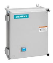
Non-reversing motor starter, Size 1, Three phase full voltage, Solid-state overload relay, OLR amp range 0.75-3.4A, 24VAC 50-60Hz coil, Non-combination type, Enclosure type 4X fiberglass, Water/dust tight noncorrosive, Standard width enclosure
