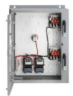
Duplex starter with alternator Size 0 Three phase full voltage Solid-state overload relay OLR amp range 5.5-22A 110VAC 50Hz / 120VAC 60Hz Coil Combination type Two 30A disconnect switches Encl NEMA type 4 painted steel Water/dust tight weather proof
