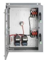
Duplex starter with alternator Size 2 Three phase full voltage Solid-state overload relay OLR amp range 13-52A 110VAC 50Hz / 120VAC 60Hz Coil Combination type Two 60A disconnect switches Enclosure NEMA type 1 Indoor general purpose use
