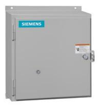
Reversing motor starter, Size 2, Three phase full voltage, Solid-state overload relay, OLR amp range 13-52A, 240V 50Hz / 277V 60Hz coil, Non-combination type, Enclosure type 4X fiberglass, Water/dust tight noncorrosive, Standard width enclosure
