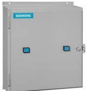
Duplex starter w/o alternator, Size 3, Three phase full voltage, Solid-state overload relay, OLR amp range 25-100A, 240V 50Hz / 277V 60Hz coil, Non-combination type, Encl NEMA type 4X 304 S-Steel, Water/dust tight noncorrosive
