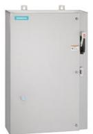
Non-reversing motor starter, Size 4, Three phase full voltage, Solid-state overload relay, OLR amp range 50-200A, 208VAC 60Hz coil, Combination type, 200A fusible disconnect, 200A/250V fuse clip, Encl NEMA type 4X 304 S-Steel, Water/dust tight noncorrosive, Standard width enclosure
