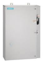
Non-reversing motor starter, Size 4, Three phase full voltage, Solid-state overload relay, OLR amp range 50-200A, Combination type, 150A circuit breaker, Encl NEMA type 4X 316 S-Steel, Water/dust tight noncorrosive, Standard width enclosure
