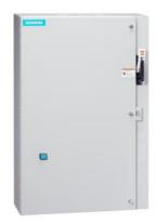
Non-reversing motor starter, Size 2 1/2, Three phase full voltage, Solid-state overload relay, OLR amp range 25-100A, 240V 50Hz / 277V 60Hz coil, Combination type, 100A circuit breaker, Enclosure NEMA type 1, Indoor general purpose use, Extra-wide enclosure
