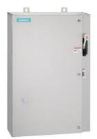
Non-reversing motor starter Size 0 Three phase full voltage Solid-state overload relay OLRelay amp range 0.75-3.4A 24VAC 50-60HZ coil Combination type 30Amp non-fusible disconnect Encl NEMA type 4X 316 S-steel Water/dust tight non-corrosive Extra-wide enclosure
