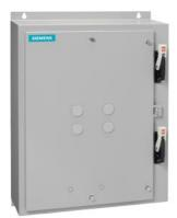
Duplex starter w/ alternator, Size 2 1/2, Three phase full voltage, Solid-state overload relay, OLR amp range 25-100A, 110V 50Hz / 120V 60Hz coil, Combination type, Two 100A circuit breakers, Enclosure NEMA type 1, Indoor general purpose use
