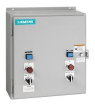
Duplex starter w/ alternator, Size 3 1/2, Three phase full voltage, Solid-state overload relay, OLR amp range 50-200A, 110V 50Hz / 120V 60Hz coil, Noncombination type, Enclosure NEMA type 1, Indoor general purpose use
