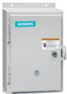
Reversing motor starter, Size 0, Three phase full voltage, Solid-state overload relay, OLR amp range 0.75-3.4A, 24VAC 50-60Hz coil, Non-combination type, Enclosure type 12, Dust/drip proof for indoors, Standard width enclosure
