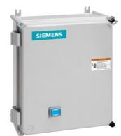
Non-reversing motor starter, Size 1, Three phase full voltage, Solid-state overload relay, OLR amp range 5.5-22A, Non-combination type, Enclosure type 4X fiberglass, Water/dust tight noncorrosive, Standard width enclosure
