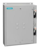
Duplex starter w/o alternator, Size 0, Three phase full voltage, Solid-state overload relay, OLR amp range 0.25-1A, 380-440/440-480V 50/60Hz coil, Combination type, Two 3A circuit breakers, Enc NEMA type 4 painted steel, Water/dust tight for outdoors
