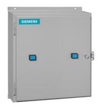
Duplex starter w/o alternator, Size 3, Three phase full voltage, Solid-state overload relay, OLR amp range 25-100A, 24VAC 50-60Hz coil, Non-combination type, Enc NEMA type 4 painted steel, Water/dust tight for outdoors
