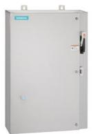
Non-reversing motor starter, Size 3, Three phase full voltage, Solid-state overload relay, OLR amp range 25-100A, 208VAC 60Hz coil, Combination type, 125A circuit breaker, Encl NEMA type 4X 316 S-Steel, Water/dust tight noncorrosive, Extrawide enclosure
