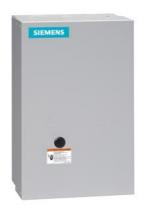
2-speed 3-phase motor starter, Size 0, One winding consequent pole, Constant or variable torque, Solid-state overload relays, Low Spd OLR range 0.75-3.4A, High Spd OLR range 0.75-3.4A, 110V 50Hz / 120V 60Hz coil, Enclosure NEMA type 1, Indoor general purpose use
