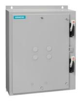
Duplex starter w/ alternator, Size 1, Three phase full voltage, Solid-state overload relay, OLR amp range 0.75-3.4A, 110V 50Hz / 120V 60Hz coil, Combination type, Two 3A circuit breakers, Enc NEMA type 4 painted steel, Water/dust tight for outdoors
