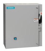
Non-reversing motor starter, Size 1 3/4, Three phase full voltage, Solid-state overload relay, OLR amp range 10-40A, 208VAC 60Hz coil, Combination type, 60A fusible disconnect, 60A/600V fuse clip, Enclosure NEMA type 1, Indoor general purpose use, Extra-wide enclosure
