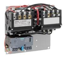
Reversing motor starter Size 2 Three phase full voltage Solid-state overload relay OLRelay amp range 13-52a 208VAC 60HZ coil Non-combination type Enclosure type (open)
